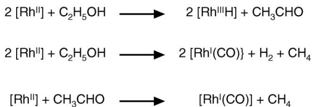
Scheme 3. Rhodium induced dehydrogenation and decarbonylation of ethanol.
